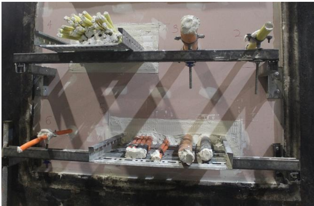
Figure 2 – Exposed face prior to test commencement
